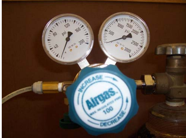
Figure 13: Two-Stage Regulator Valve.
